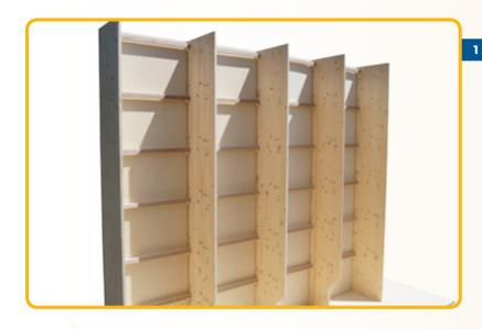
If the box is delivered with a rear panel, insert the panel in the grooves at the back of the side panels. Then, from the top to the bottom, push the rear crossbars with the dimensions 19 x 27 mm onto the metal bolts on the side panels. 5 bars in total.
