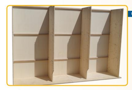
If the box is delivered with a rear panel, insert the panel in the grooves at the back of the side panels. Then, from the top to the bottom, push the rear crossbars with the dimensions 19 x 27 mm onto the metal bolts on the side walls. 4 bars in total. In doing so, the holes can also point to the back as they are not needed for breeding boxes.
