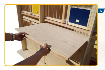
Insert the droppings floors. Afterwards, accurately align the box vertically and horizontally using the spirit level and screw it securely to the back wall.
